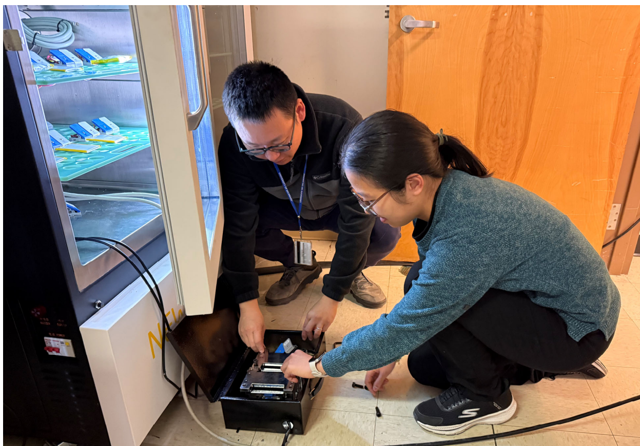
Fig. 2. Researchers prepare and instrument battery-test hardware to examine how real-world electrical and mechanical conditions influence battery safety in space-relevant environments.
