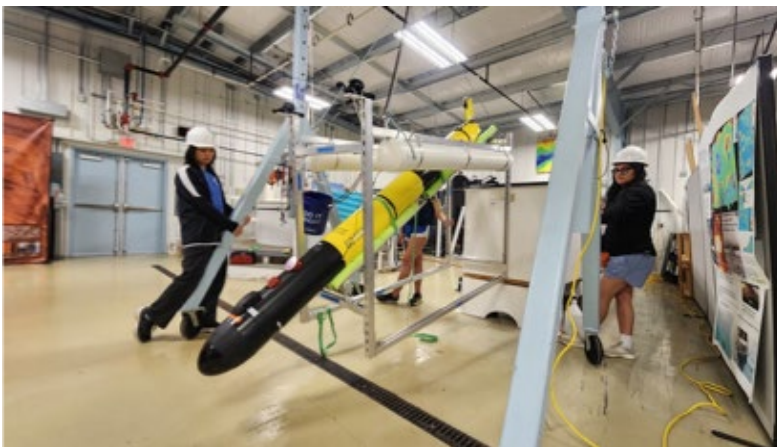
PHOTO CAPTION: An autonomous glider is prepared to take in situ underwater measurements.
