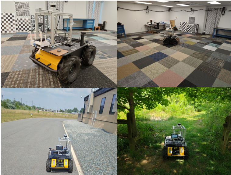
Figure 1: We validate our navigation and perception algorithms in different indoor and outdoor environments on UD campus with a Husky vehicle equipped with low-cost, low-fidelity LiDAR, camera and inertial sensors. These technologies can be translated to autonomous landing of a spacecraft in planetary exploration missions.
