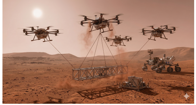
Figure 1: Illustration of multi-UAV cooperative aerial manipulation and load transportation in planetary exploration scenarios.
