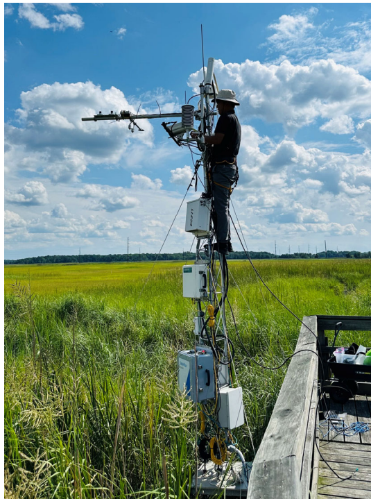
Figure 3. Stereo camera installation on a salt marsh monitoring tower at the St. Jones Reserve.
